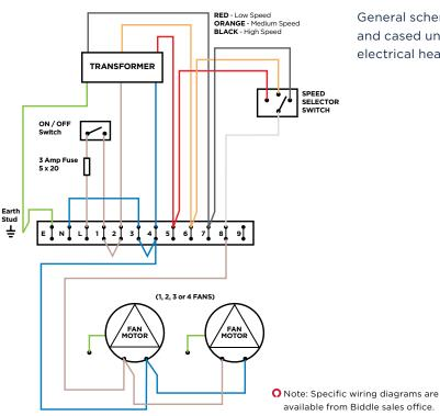
General schematic for chassis and cased units (does not include electrical heating options).
